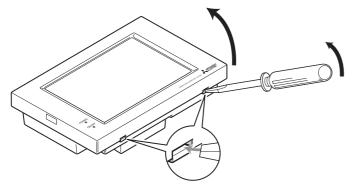
Insert a flat-tip screwdriver in the holes indicated and move the handle up to remove the cover.
