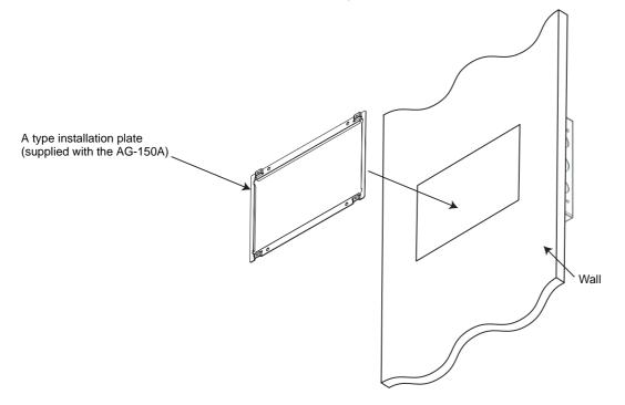
(2) Screw the A type installation plate down by putting the M4 flathead screws (supplied with AG-150A) through the mounting holes on the Electric Box.
