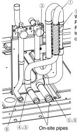
Wrap the pipe cover here. Fix compressor cables to Pipe cover with Cable tie to keep them out of direct contact with the pipes.
