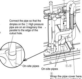
Wrap the pipe cover here. Fix compressor cables to Pipe cover with Cable tie to keep them out of direct contact with the pipes.
