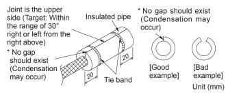
4. Wrap the tape for piping construction around the joint between the insulated pipe and the field refrigerant piping to prevent the insulated joint from being exposed.
