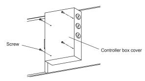
Install a PG connection or the like, then connect the power supply cable to the TM1 terminal block.
