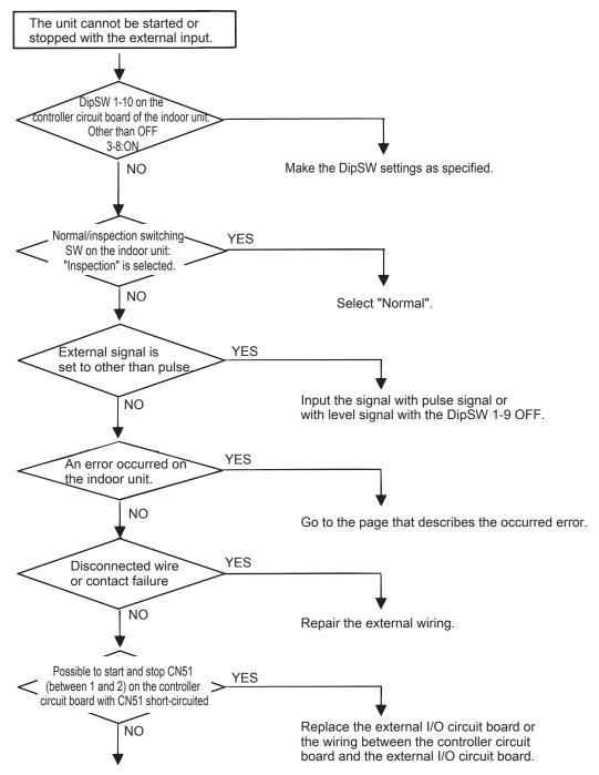
Replace the controller circuit board.
