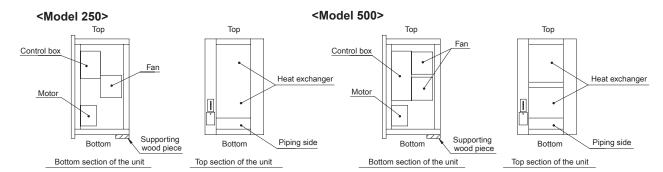
To put the top and bottom sections of the unit together, follow the procedures above in the reverse order.
