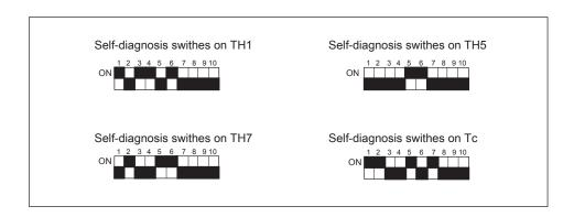
Use these switches to figure out the values of TH1, Tc - TH5, and Tc - TH7.
