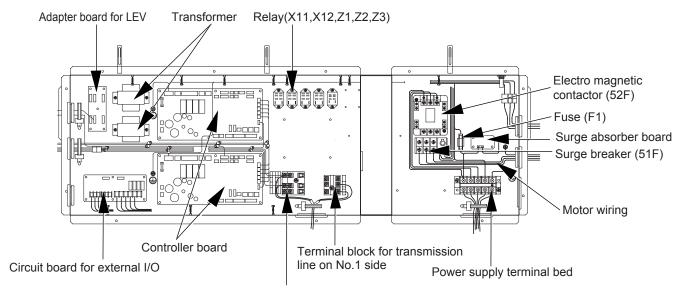
Terminal block for transmission line on No.2 side (upper) Terminal block for MA remote controller (lower)
