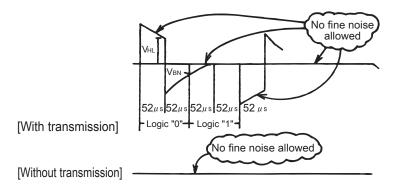
Check the wave pattern of the transmission line with an oscilloscope. The following conditions must be met.
