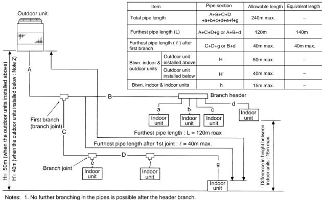
When cooling operation is performed when the outdoor temp. is 0°C or lower : H'= 4m or less.
