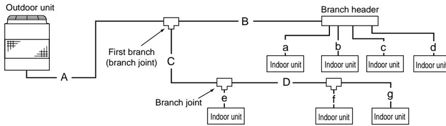
(2) In the case of replacing a typical split system
