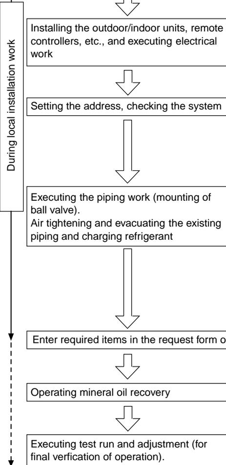
It is necessary to charge refrigerant in a rated quantity and adjust the quantity. Be sure to execute when the piping length is unknown. For detail, consult the agent of your dealer.
