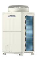
The City Multi Y Series makes use of a two pipe refrigerant circuit throughout, with branch pipes feeding indoor units, allowing manual changeover from cooling to heating to ensure that a constant indoor climate is maintained.
