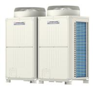
The City Multi Y Series makes use of a two pipe refrigerant circuit throughout, with branch pipes feeding indoor units, allowing manual changeover from cooling to heating to ensure that a constant indoor climate is maintained.
