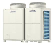
The City Multi Y Series makes use of a two pipe refrigerant circuit throughout, with branch pipes feeding indoor units, allowing manual changeover from cooling to heating to ensure that a constant indoor climate is maintained.
