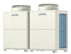
The City Multi Y Series makes use of a two pipe refrigerant circuit throughout, with branch pipes feeding indoor units, allowing manual changeover from cooling to heating to ensure that a constant indoor climate is maintained.
