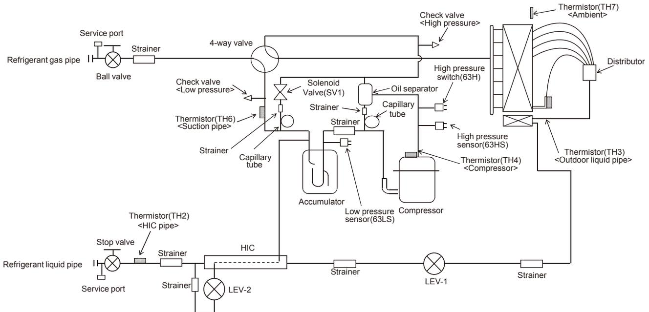
Capillary tube for oil separator :  $\phi 2.5 \times \phi 0.8 \times L800$
