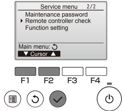
② Select "Remote controller check" from the Service menu, and press the
