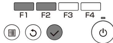
② Select "Test run" with the **F1** or **F2** button, and press the button.
