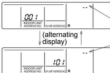
"-" will appear in the unit type display location when an address has been cleared normally.
