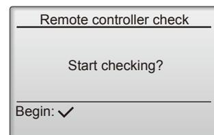
Check the remote controller display and see if anything is displayed (including lines). Nothing will appear on the remote controller display if the correct voltage (8.5–12 V DC) is not supplied to the remote controller. If this is the case, check the remote controller wiring and indoor units.
