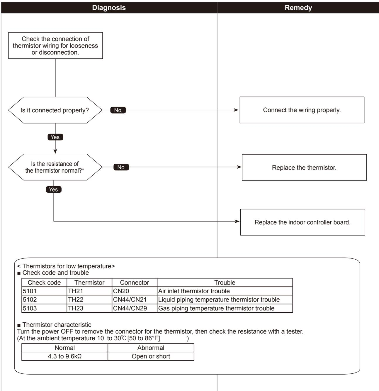
\* Symbols for thermistors and connectors may be different depending on the model. Please refer to its wiring diagram.
