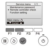
② Select "Remote controller check" from the Service menu, and press the 🔾 button to start the remote controller check and see the check results.
