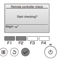
3 **OK:** No problems are found with the remote controller. Check other parts for problems.
