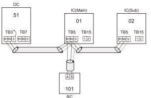
Multiple indoor units operated together by 1 remote controller
