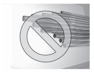
Both ends of the pipes should be sealed until just before brazing. Keep elbows and T-joints wrapped in plastic bags to keep dust, dirt, and moisture out.
