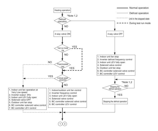
\*Note 1. When the outdoor unit goes into the defrost mode, defrost command is sent to the BC controller and indoor units.
