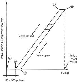
\*When the power is turned on, the valve closing signal of 2200 pulses (Indoor LEV, BC controller LEV1 (G1 type only), and LEV3), or 3200 pulses (BC controller LEV1 (GA1 type only)), will be output from the indoor board to LEV to fix the valve position. It must be fixed at point (A)
