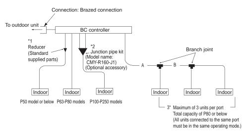
The ports of the BC controller accommodates the pipes on P63-P140 models of indoor units. To connect other types of indoor units, follow the procedure below.
