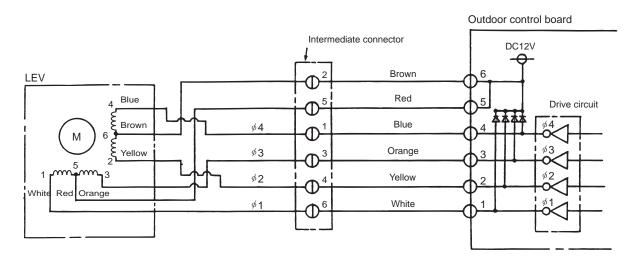
Note. The connector numbers on the intermediate connector and the connector on the control board differ. Check the color of the lead wire to judge the number.
