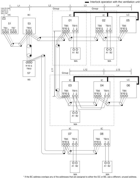
If the BC address overlaps any of the addresses that are assigned to either the OC or BS, use a different, unused address. OC, and BS addresses (lowest indoor unit address in the group plus +50) have higher priority than the BS address.
