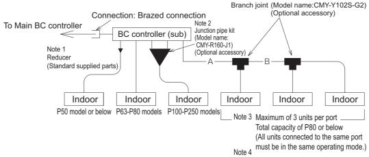
Note 4 Group the indoor units together that connected to the same port if multiple indoor units are connected to the same port on BC controller. Also share one thermo-stat such as on remote controller so that they turn on/off at the same time.
