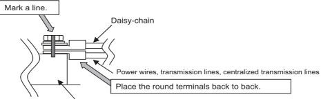
Power supply terminal block, indoor-outdoor transmission line terminal block, and centralized controller transmission line
