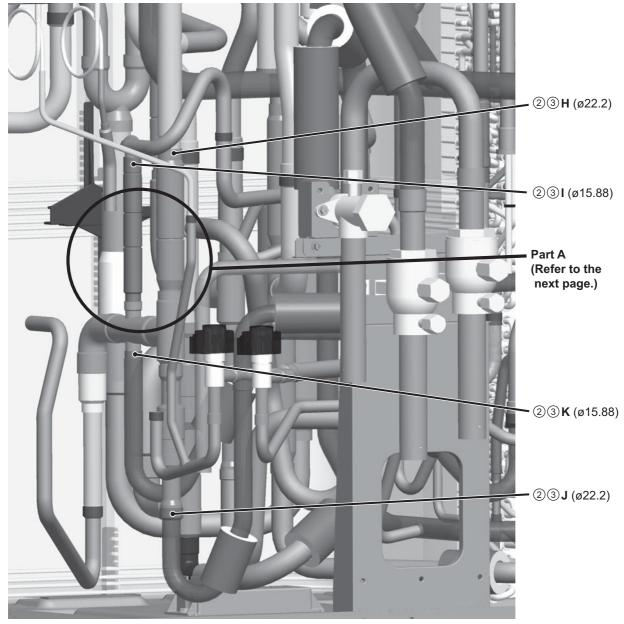
\* After removing Solenoid valve block ASSY
