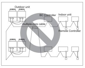
TB3: Terminal block for indoor-outdoor transmission line TB7: Terminal block for centralized control
