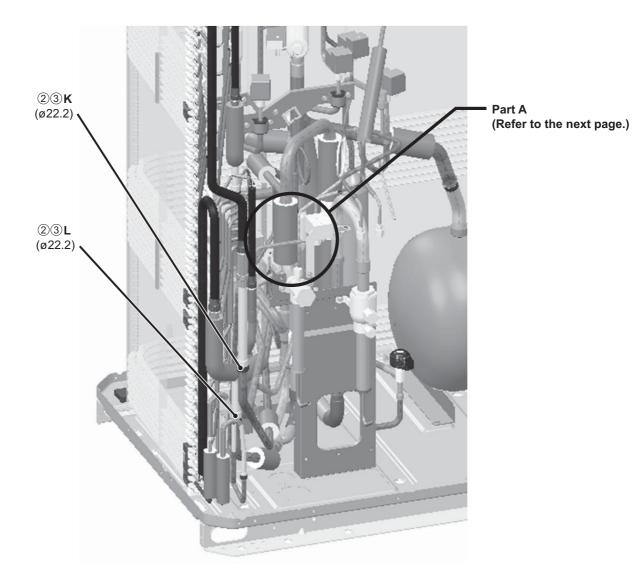
\* After removing Solenoid valve block ASSY
