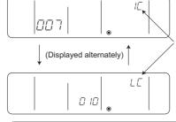
If registration is successfully completed, the two displays as shown on the left will appear alternately.
