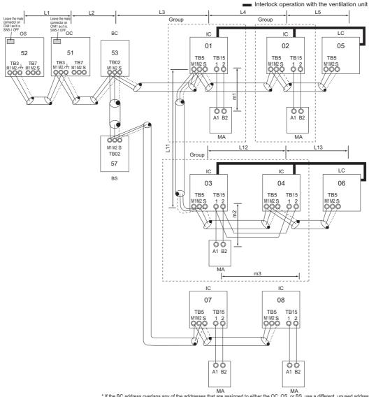
If the BC address overlaps any of the addresses that are assigned to either the OC, OS, or BS, use a different, unused address OC, OS, and BS addresses (lowest indoor unit address in the group plus +50) have higher priority than the BS address.
