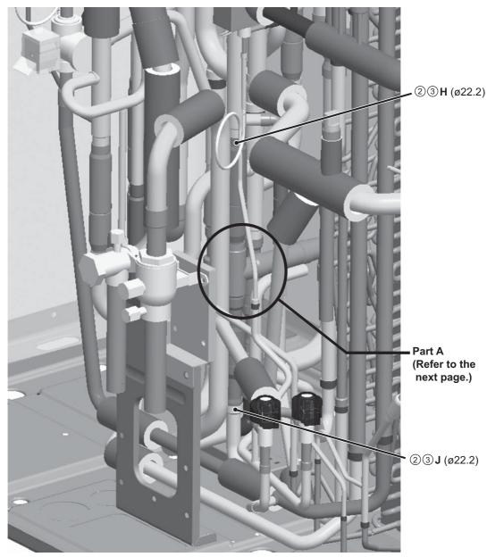
\* After removing Solenoid valve block ASSY
