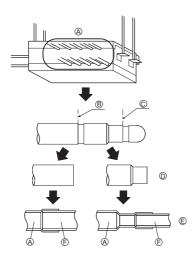
Be sure to have pipe expansion of indoor unit connecting port by cutting the piping at the cutting point which depends on the indoor unit capacity.
