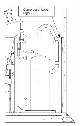
5. Remove the compressor wires, compressor cover, and the right.
