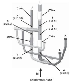
When replacing CV4a: Remove the brazing 1.
