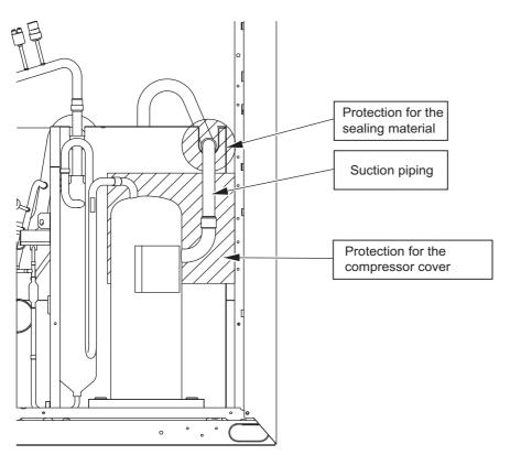
Place protective materials on the insulation lining of the compressor cover and on the sealing material on the compressor suction pipe to protect them from the torch flame, debraze the pipe, and replace the compressor.
