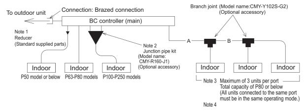
Note 4 Group the indoor units together that connected to the same port if multiple indoor units are connected to the same port on BC controller. Also share one thermo-stat such as on remote controller so that they turn on/off at the same time
