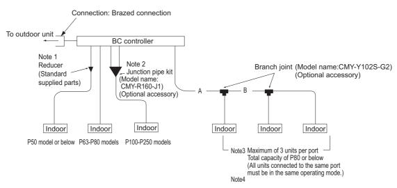
Note 4 Group the indoor units together that connected to the same port if multiple indoor units are connected to the same port on BC controller. Also share one thermo-stat such as on remote controller so that they turn on/off at the same time.
