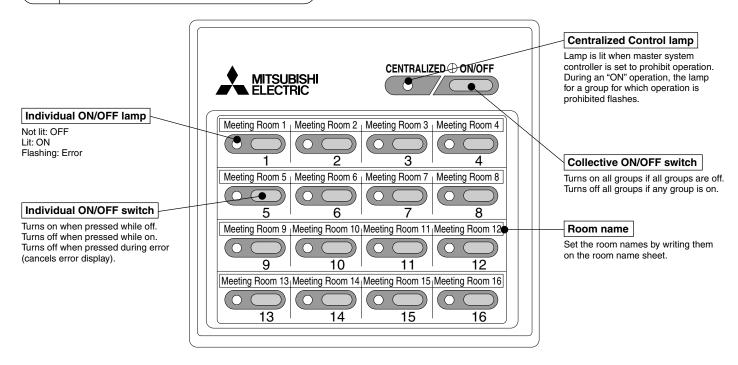
NOTE • If ON/OFF operation is prohibited by another system controller, the prohibited group's Individual ON/OFF button and the Collective ON/OFF switch cannot be operated. When this operation is attempted, the Under Central Control lamp will flash twice.
