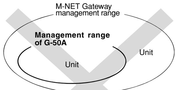
When G-50A controls another system controller or when the system contains only G-50A:
