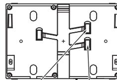
External input adapter cable access hole External output adapter cable access hole
