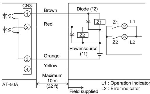
Use relays that meet the following specifications for relays indicated as Z1 and Z2 in the figure.
