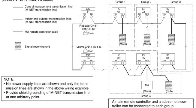
① Wiring from signal receiving unit.
