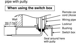
• When opening a hole using a drill for Signal Receiving Unit cord (or taking the cord out of the back of the Signal Receiving Unit), seal that hole
