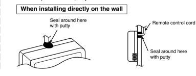
(5) Install the lower case on the switch box or directly on the wall.
