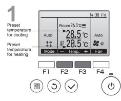
The current preset temperatures will appear. Press the F2 or F3 button to display the Settings screen.
