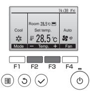
Press the F2 button to decrease the preset temperature, and press the F3 button to increase.
