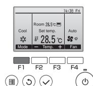
Press the F1 button to go through the operation modes in the order of "Cool, Dry, Fan, Auto, and Heat." Select the desired operation mode.
