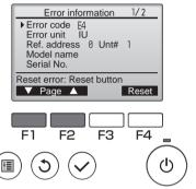
Error code, error unit, refrigerant address, unit model name, and serial number will appear. The model name and serial number will appear only if the information have been registered.
