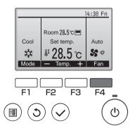
Press the F4 button to go through the fan speeds in the following order.
