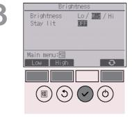
Adjust the brightness with the F1 or F2 button. "ON" or "OFF" can be selected for the "Stay lit" setting with the F4 button.
