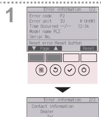
Error code, error unit, refrigerant address, unit model name, date and time on which an error occurred, and serial number will appear.
