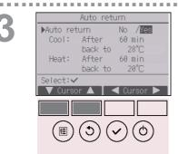
The screen to make the settings for the automatic return to the preset temperature will appear.
