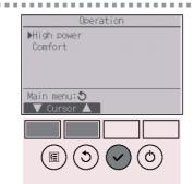
Select "High power" from the Operation menu during Cooling, Heating, or Auto operation, and press the SELECT button.
