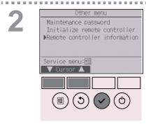
Move the cursor to "Remote controller information" with the F1 or F2 button, and press the SELECT button.
