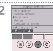
Move the cursor to "Brightness" with the F1 or F2 button, and press the SELECT button.
