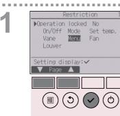
To enable the operation lock function, set the item "Operation locked" to "Yes".
