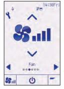
Each pressing of the  $\bigtriangledown$  or  $\blacktriangle$  button cycles through the following fan speeds.
