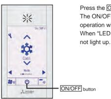
Press the ON/OFF button. The ON/OFF lamp will light up in green, and the operation will start. When "LED lighting" is set to "No," the ON/OFF lamp will
