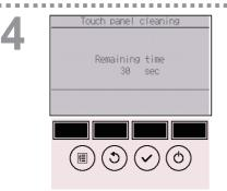
This screen allows the user to wipe the touch panel for 30 seconds without accidentally changing the settings.
