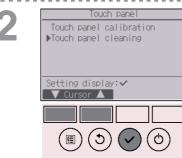
Move the cursor to "Touch panel cleaning" with the F1 or F2 button, and press the SELECT button.
