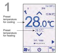
The current preset temperatures will appear. Each pressing of the  $\blacksquare$  or  $\blacktriangleright$  button switches the preset temperatures for cooling and heating.
