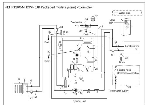
To enable draining of the cylinder unit an isolating valve should be positioned on both the inlet and outlet pipework. No valve should be fitted between the expansion valve (item 35) and the cylinder unit (safety matter).
