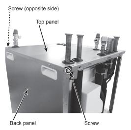
The photo shows the left side. The opposite side also has the screw to be removed on the same position.
