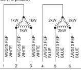
Measure the resistance between the terminals with a tester.
