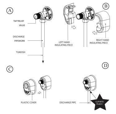
Fig 7 - Schematic installation diagram
