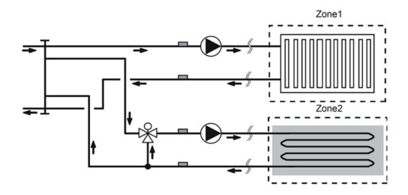
Fig 14 - Optional 2 zone twin temperature control pack - component wiring
