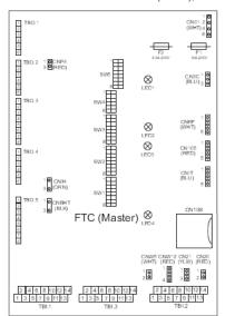
When the wires are wired to adjacent terminals use ring terminals and insulate the wires.
