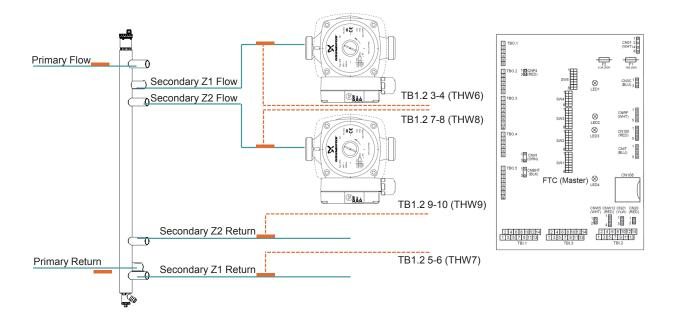
Fig 12 - 2 zone control pack - dip switch settings
