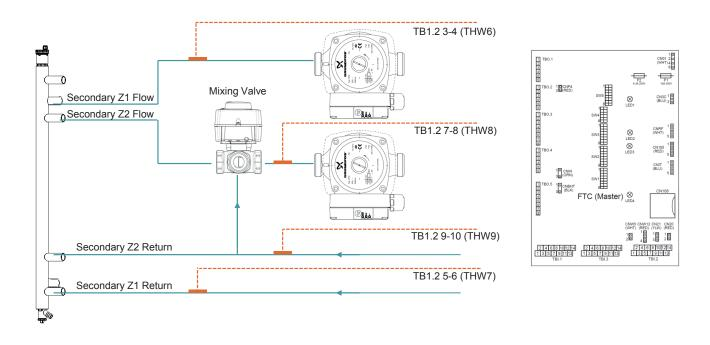
Fig 16 - Optional 2 zone twin temperature control pack - dip switch settings
