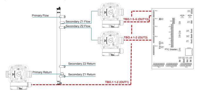
Fig 11 - 2 zone control pack - temperature sensor wiring
