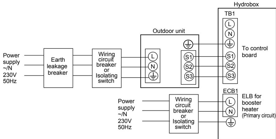
\* Installer MUST affix label A that is included with the manuals near each wiring diagram for hydrobox and outdoor units.
