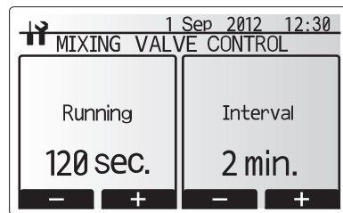
Mixing valve setting screen
