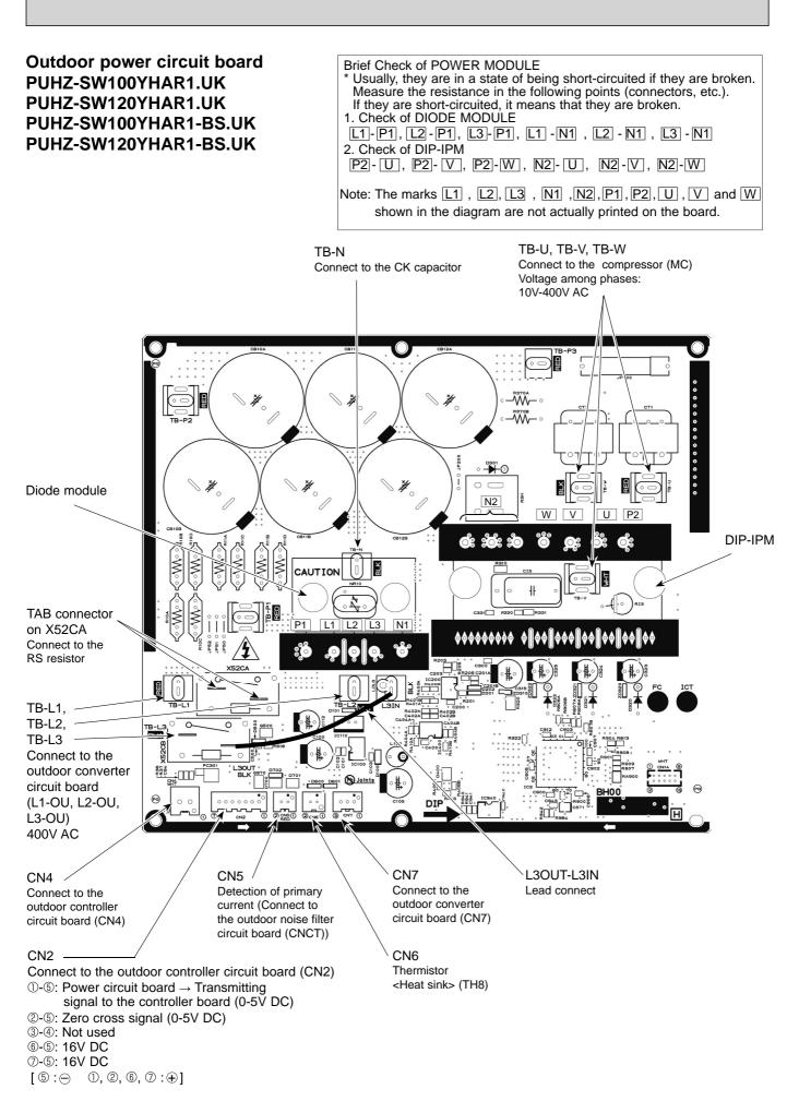
Outdoor converter circuit board PUHZ-SW100YHA.UK PUHZ-SW120YHA.UK PUHZ-SW100YHAR1.UK PUHZ-SW120YHAR1.UK
