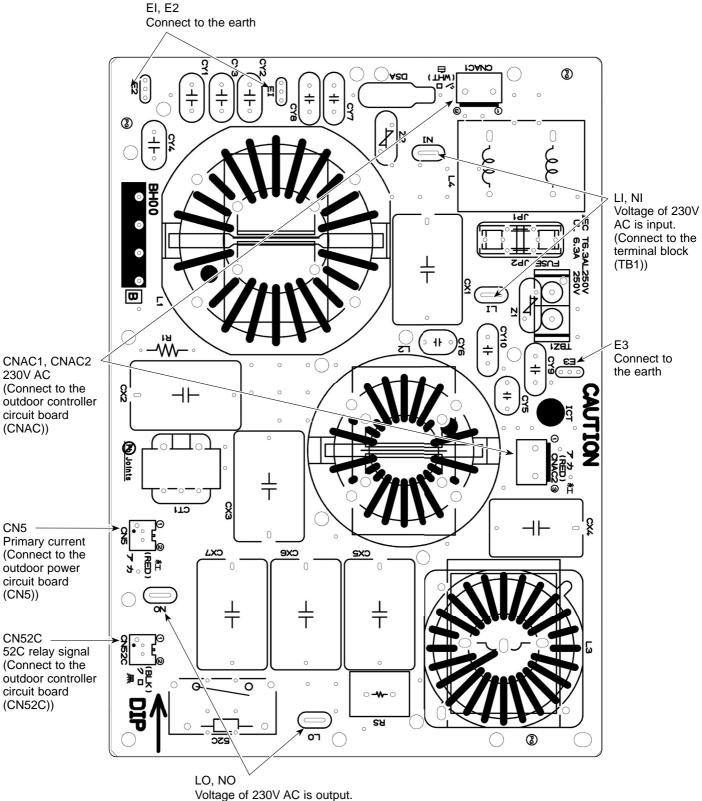
Voltage of 230V AC (Connect ACL)
