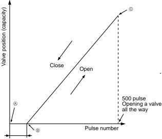
Opening a valve :  $8 \rightarrow 7 \rightarrow 6 \rightarrow 5 \rightarrow 4 \rightarrow 3 \rightarrow 2 \rightarrow 1 \rightarrow 8$ Closing a valve :  $1 \rightarrow 2 \rightarrow 3 \rightarrow 4 \rightarrow 5 \rightarrow 6 \rightarrow 7 \rightarrow 8 \rightarrow 1$ The output pulse shifts in above order.
