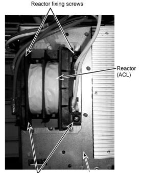
Reactor fixing screws
