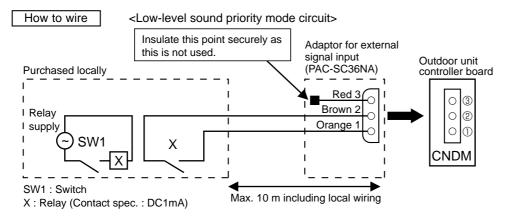
1) Make the circuit as shown above with Adaptor for external signal input (PAC-SC36NA).
