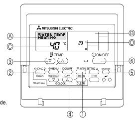
(1) Press the (INITIAL SETTING♥) button ① for 3 seconds to activate the initial setting mode.
