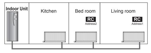
\* The above figure shows the examples when the living room is set as a target room RC 1 (wireless remote controller 1), and when the bed room is set as a target room RC 2 (wireless remote controller 2).
