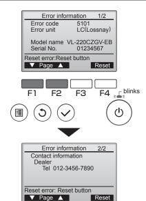
Error code, error unit, unit model name, and serial number will appear.
