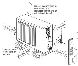
When the piping is to be attached to a wall containing metals (tin plated) or metal netting, use a chemically treated wooden piece 20 mm or thicker between the wall and the piping or wrap 7 to 8 turns of insulation vinyl tape around the piping.
