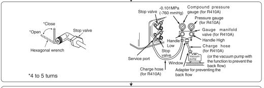
Remove the gauge manifold valve quickly from the service port of the stop valve.
