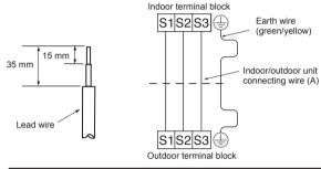
Make earth wire a little longer than others. (More than 55 mm) For future servicing, give extra length to the connecting wires.
