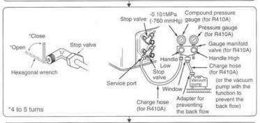
Remove the gauge manifold valve quickly from the service port of the stop valve.
