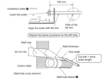
Be sure to use wall hole sleeve **©** to prevent the outdoor connecting wires from contacting with metal part in the wall and to prevent damage by rat in case the wall is hollow.
