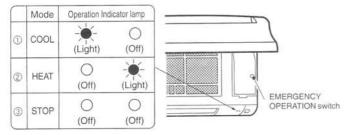
In starting the heating operation, indoor unit fan may not operate to prevent blowing cool air. Please wait for a few minutes until the temperature of heat exchanger rises
