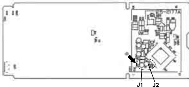
**NOTE :** For remodelling, take out the batteries and press the OPERATE/STOP(ON/OFF)button twice or 3 times at first. After finish remodelling, put back the batteries then press the RESET button.
