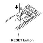
NOTE1: If the RESET button is not pressed, the remote controller may not operate correctly.
