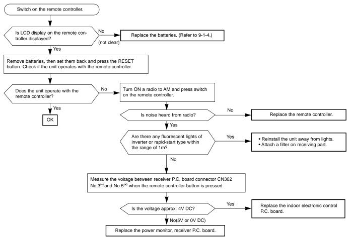
The unit doesn't operate with the remote controller.
