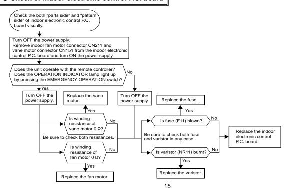
When OPERATION INDICATOR lamp flashes 0.5-second intervals or 1-time. Outdoor unit does not operate.
