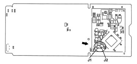
The P.C. board has the print "J1" and "J2". Solder "J1" and "J2" according to the number of indoor unit as shown in Table 1. After modification, press the RESET button.
