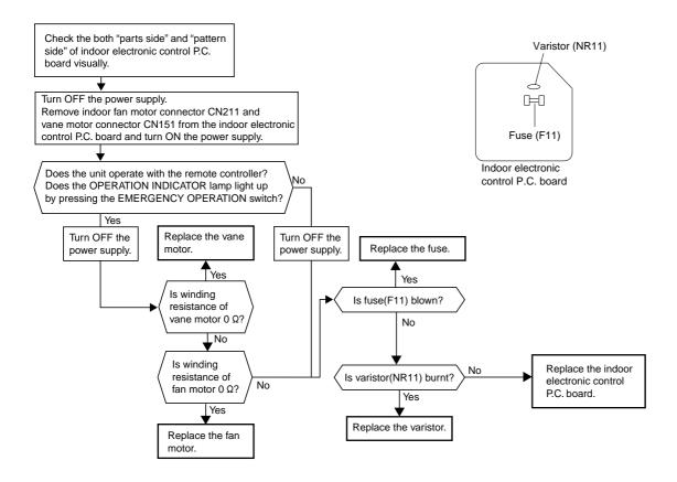
When OPERATION INDICATOR lamp flashes ON and OFF in every 0.5-second. Outdoor unit doesn't operate.
