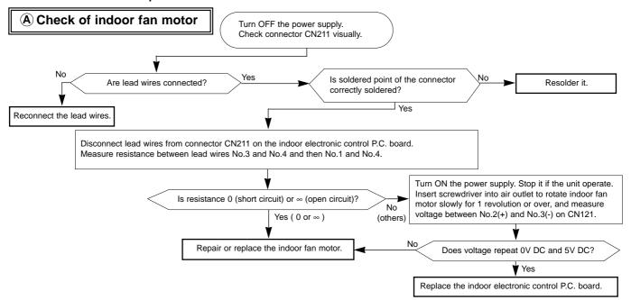
Indoor unit operates by pressing the EMERGENCY OPERATION switch, but doesn't operate with the remote controller.
