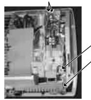
Screw of the electrical cover Screw of the electrical box
