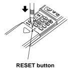
NOTE: If the RESET button is not pressed, the remote controller may not operate correctly.
