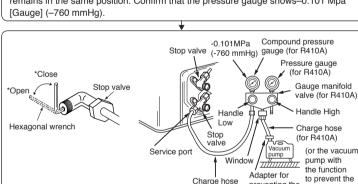
preventing the back flow) (for R410A) \*4 to 5 turns Remove the gauge manifold valve guickly from the service port of the stop valve.
