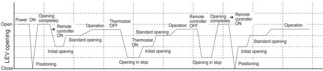
**NOTE**: Opening increases and decreases to be in the target discharge temperature during operation.
