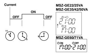
**NOTE:** If the main power is turned OFF or a power failure occurs while ON/OFF timer is active, the timer setting is cancelled. As these models are equipped with an auto restart function, the air conditioner starts operating with timer cancelled when power is restored.
