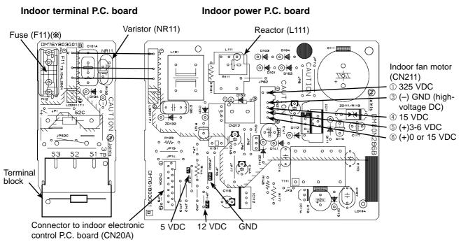
\* Please replace the fuse after removing the indoor terminal P.C. board from the electrical box.
