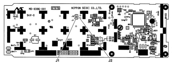
The P.C. board has the print "J1" and "J2". Solder "J1" and "J2" according to the number of indoor unit as shown in Table 1. After modification, press the RESET button.
