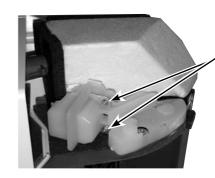
Screws of the vertical vane motor unit cover
