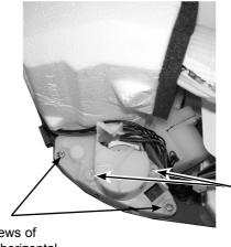
Screws of the horizontal vane motor unit Screws of the horizontal vane motor unit cover
