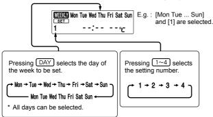
(3) Press (N/OFF), ( and ), and ( buttons to set ON/OFF, time, and temperature.
