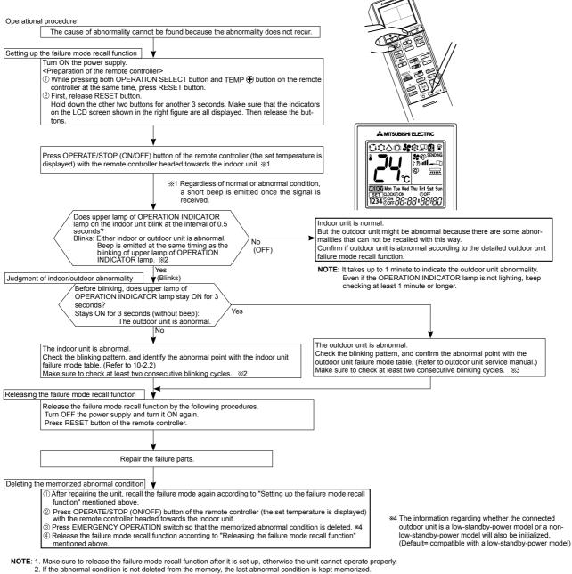
$\frak{\%}2$ . Blinking pattern when the indoor unit is abnormal:
