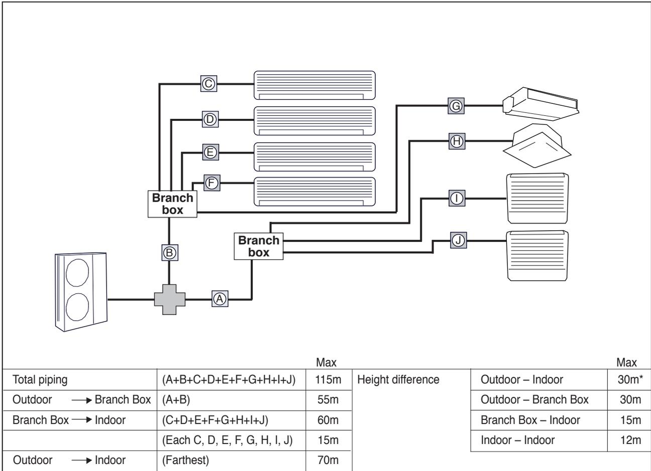
\* In case of installing outdoor unit higher than indoor unit : 20m
