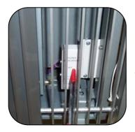
Reset the Filter Dirty Indicator after cleaning by a quick press of the Reset Button (even if the indicator has not gone red).
