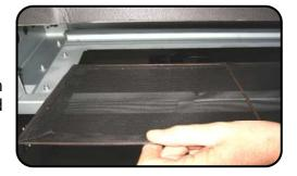
Refit the filters opposite to removal. The filters are very durable but may need to be replaced after a number of service intervals.
