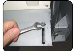
grille core is fitted and tighten the bolts (see photo and Figure 1). It is necessary to temporarily fit the grille core to gauge the required height of the air separator plate(s).
