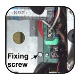
The Interface PCB on its mounting plate is held in place by a screw located at the left-hand side of the board. Remove the fixing screw and carefully slide the pcb fully out.
