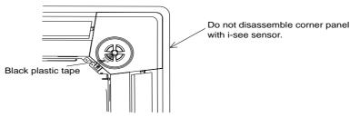
i-see sensor (At the ambient temperature of 10°C~40°C)
