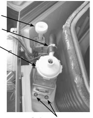
Drain pump assembly fixing screw
