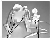
Drain pump fixing screw
