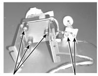
Drain pump fixing screw
