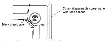
i-see sensor (At the ambient temperature of  $10^{\circ}\text{C} \sim 40^{\circ}\text{C}$ )
