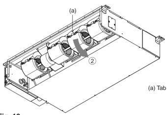
3. Removing the motor cable
