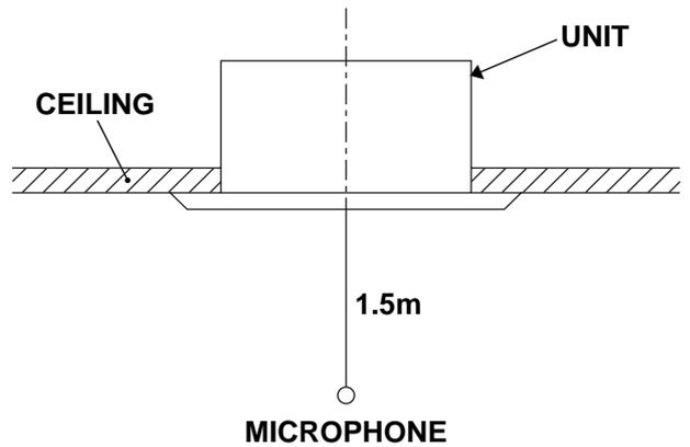
**NOTE:** The sound level is measured in an anechoic room where echoes are few, when compressor stops. The sound may be bigger than the indicated level in actual use due to surrounding echoes. The sound level can be high by about 2 dB than the indicated level during cooling and heating operation.
