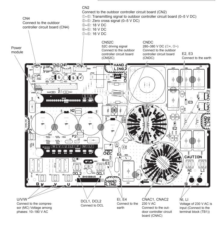
Outdoor power circuit board PUHZ-ZRP100YKA3.UK PUHZ-ZRP125YKA3.UK PUHZ-ZRP140YKA3.UK PUHZ-ZRP200YKA2.UK PUHZ-ZRP250YKA2.UK
