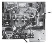
Noise filter circuit board (N.F.)
