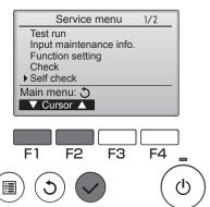
2 With the  $\fbox{F1}$  or  $\fbox{F2}$  button, enter the refrigerant address, and press the  $\textcircled{\checkmark}$  button.
