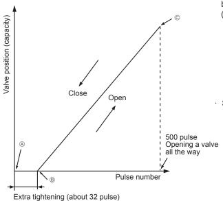
· When the power is turned on, 700 pulse closing valve signal will be sent till it goes to @ point in order to define the valve position. (The pulse signal is being sent for about 20 seconds.)
