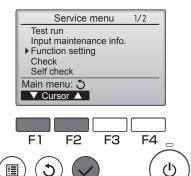
② Set the indoor unit refrigerant addresses and unit numbers with the F1 through F4 buttons, and then press the button to confirm the current setting.
