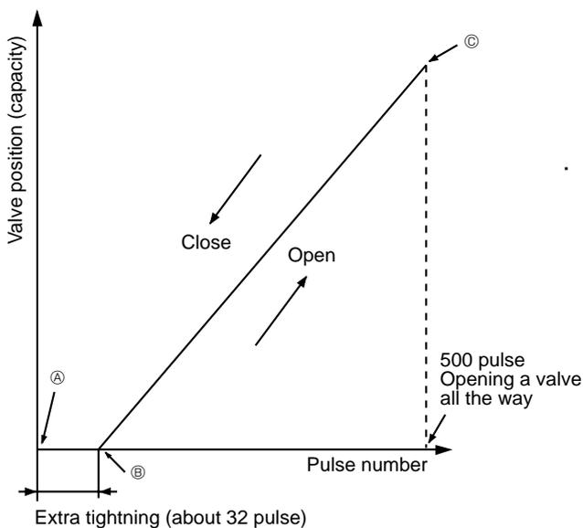
When the valve moves smoothly, there is no sound or vibration occurring from the linear expansion valve : however, when the pulse number moves from ㉞ to ㉟ or when the valve is locked, sound can be heard.
