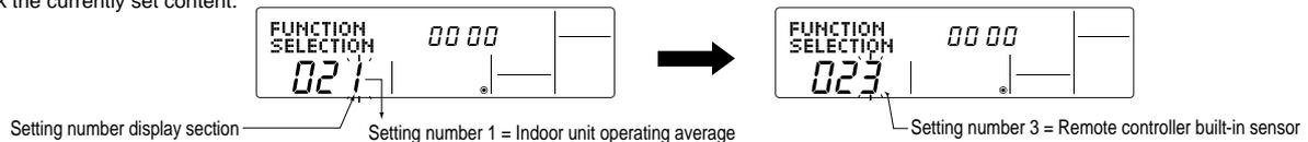
Ⓒ Press the [**TEMP**] buttons (**(▽)** and **(△)**) to select the desired setting number.
