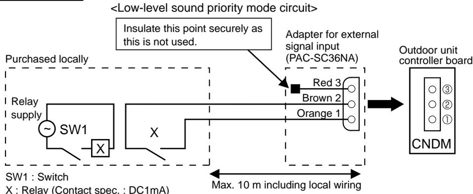
1) Make the circuit as shown above with adapter for external signal input(PAC-SC36NA).
