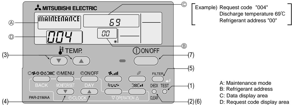
(1) Press the **TEST** button for 3 seconds so that [ Maintenance mode] appears on the screen (at A).
