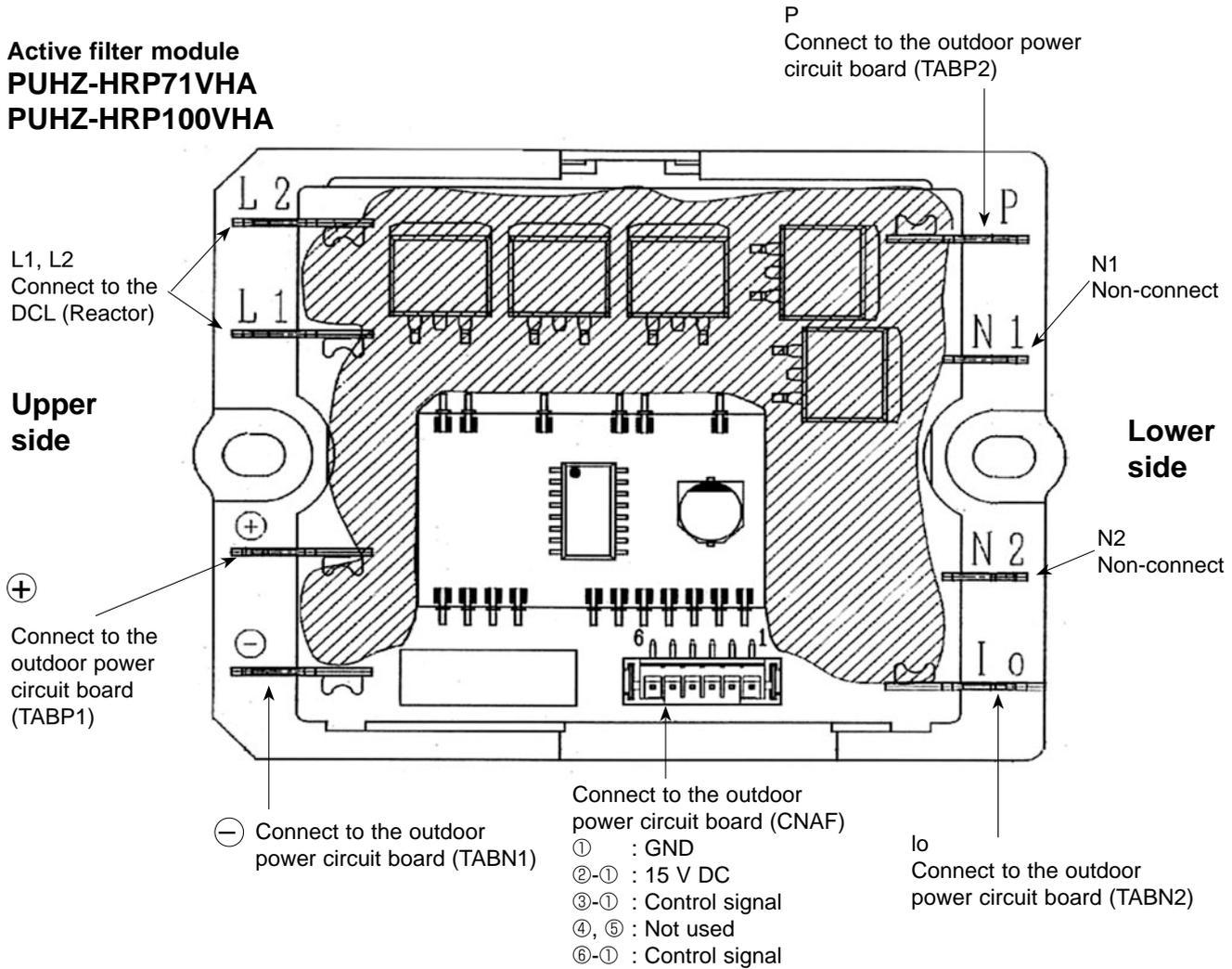
**Connection and internal circuit diagram**
