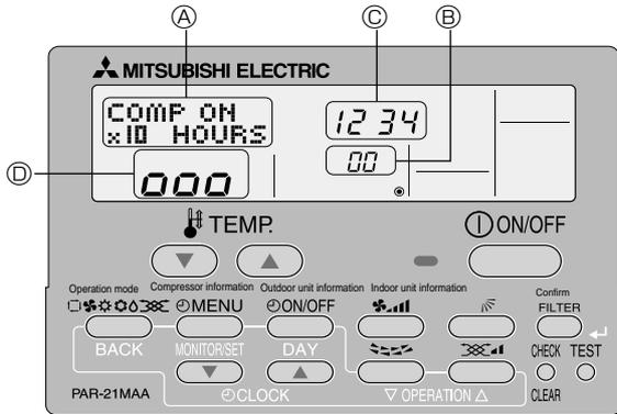
This air conditioner (Outdoor unit) can detect refrigerant leakage which may happen during a long period of use. In order to enable the leakage detection, the following settings are required to let the unit memorize the initial condition (initial refrigerant amount).
