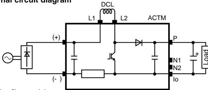
**Tester check points of Active filter module**
