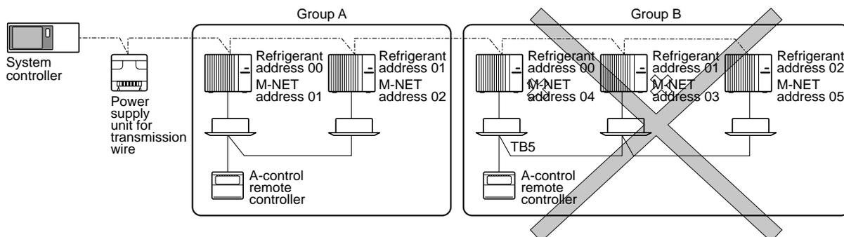
\* In group B, M-NET address of the outdoor unit whose refrigerant address is "00" is not set to the minimum in the group. As "3" is right for this situation, the setting is wrong. Taking group A as a good sample, set the minimum M-NET address in the group for the outdoor unit whose refrigerant address is "00".
