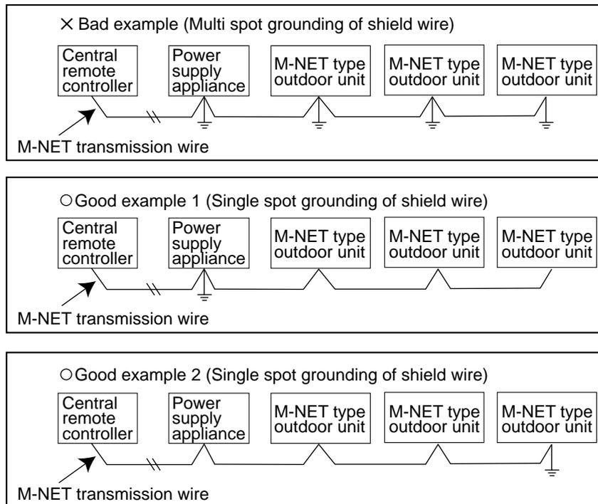
If there are more than 2 grounding spots on the shield wire, noise may enter into the shield wire because the ground wire and shield wire form one circuit and the electric potential difference occurs due to the impedance difference among grounding spots. In case of single spot grounding, noise does not enter into the shield wire because the ground wire and shield wire do not form one circuit.
